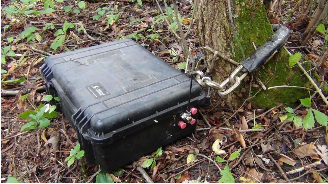
Figure B.1. ATS datalogger setup with a Lotek UHF antenna, being used for detecting VHF-collared coyotes during novel object testing.
