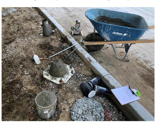
**Main Duty: Preparing and Testing Concrete**
